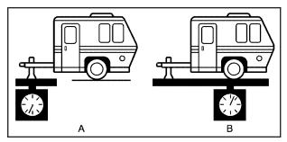
The trailer tongue weight (A) should be 10 percent to 15 percent of the total loaded trailer weight (B), up to a maximum of 400 lbs (181 kg) with a weight carrying hitch.
